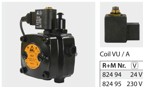
Pump VU. Single line intake or double line intake. Cable 700 mm. Pressure adjustable 6 - 18 bar
