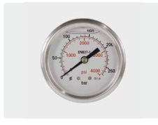
Ø 50 mm. 1/4" M. Housing stainless steel. Inlet at the back
