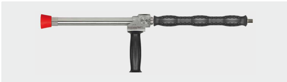
1/4" M. Stainless steel. Longcast lance 350 mm with insulation ST-29 Cool & Compact 330 mm, grip aside and nozzle protector made out of plastic without nozzle. Max. 280 bar / 130 l/min / 100 °C
