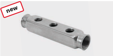
Stainless steel. 2 x 3 connections. H x W x D: 36 x 193 x 40 mm. 290 g. Max. 10 bar. 150 °C
