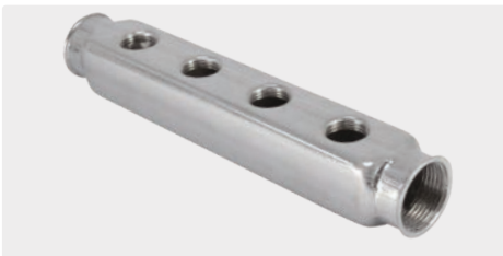
Stainless steel. 4 connections. H x W x D: 36 x 243 x 40 mm. 390 g. Max. 10 bar. 150 °C
