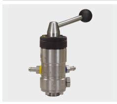
3/8" F: 1/2" F: 2 x hose tail 9 mm. The chemical dosing is adjusted by 2 x 10 exchangeable nozzle inserts (0.5 - 1.5 mm). Max. 350 bar / 100 °C
