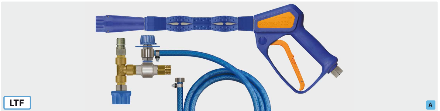
easywash365+ foam set: easywash365+ foam lance standard with foam head ST-75, injector ST-160 (Coupling ST-45-250 nickel-plated brass, plug ST-45-250 zinc-plated steel and M22 M) with metering valve ST-161, suction hose 1000 mm and suction filter ST-32. Max. 250 bar / 90 °C
