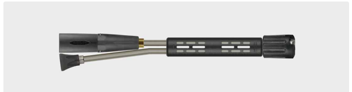
Twin foam lance with vented handle ST-9 205 mm, change-over valve ST-58, nozzle protector ST-10 without nozzle and foam head ST-75.1 without nozzle. A foam injector is required. Max. 350 bar / 45 l/min / 100 °C
