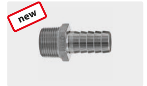
Hose barb 3/4" M. 60° cone. Stainless steel. Max. 15 bar
