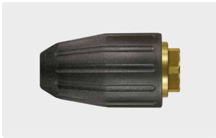
1/4" F. Spray angle 20°. 200 - 350 bar. Max. 100 °C
