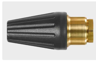
1/2" F. Spray angle 20°. 120 - 250 bar. Max. 100 °C
