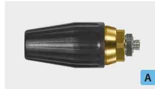
1/8" M. Spray angle 20°. 100 - 250 bar. Max. 100 °C
