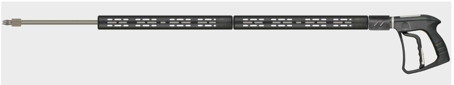
Professional steam gun ST-4000 weep version with lance stainless steel, vented handle ST-9 380 mm and steam low pressure nozzle made out of stainless steel. Max. 20 bar / 200 °C
