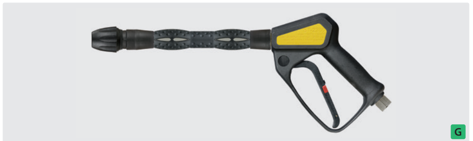
Professional gun with extension ST-9.1 260 mm and coupling KW. Max. 310 bar / 45 l/min / 150 °C
