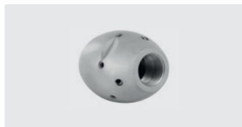
3/8" F. 6x 75° 3x 30° +1x 0°. 30-100 l/min. For \text{R} \text{D} 100-200 mm. Outside \text{D} 35 mm. \text{G} 314 g.
