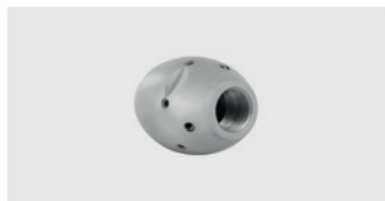
1/4" F. 6x 75° 3x 30° +1x 0°. 25-70 l/min. For \text{R} \text{D} 75-150 mm. Outside \text{D} 30 mm. \text{G} 223 g.
