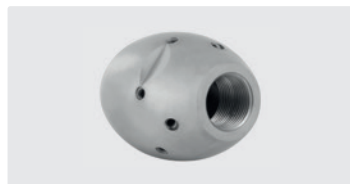
1/2" F. 6x 75° 3x 30° +1x 0°. 80-140 l/min. For \text{R} \text{D} 120-250 mm. Outside \text{D} 40 mm. \text{G} 630 g.
