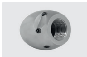
3/4" F. 6x 75° +1x 0°. 30-100 l/min. For \text{R} \text{D} 120-250 mm. Outside \text{D} 50 mm. \text{G} 567 g.
