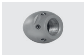
3/8" F. 6x 75° +1x 0°. 25-70 l/min. For \text{R} \text{D} 75-150 mm. Outside \text{D} 35 mm. \text{G} 207 g.
