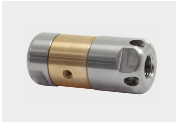
1/4" F. 4 rear jets. 3 side jets. Outside \varnothing 30 mm. ☒ 314 g.
