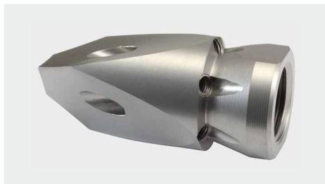
350 bar. 1/2" F. \square 68 mm, \varnothing = 31 mm, \boxplus 0.17 kg. For tubes > 60 mm. Lateral front jets with hardened stainless steel nozzle inserts
