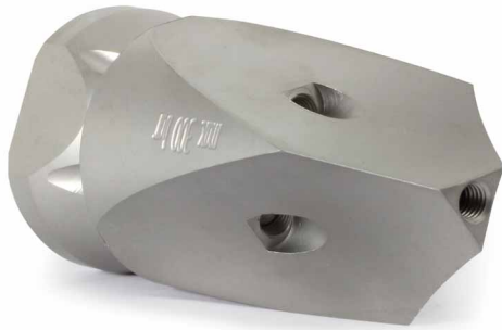
350 bar. 1/4" F. \square 50 mm, \varnothing = 25 mm, \boxplus 0.13 kg. For tubes > 30 mm. Lateral front jets 0.5 mm drilled
