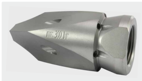
300 bar. 3/4" F. \square 80 mm, \varnothing = 38 mm, \boxplus 0.29 kg. For tubes > 60 mm. Lateral front jets with hardened stainless steel nozzle inserts
