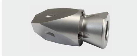
350 bar. 1/4" F. \square 50 mm, \varnothing = 25 mm, \boxplus 0.13 kg. For tubes > 30 mm. Lateral front jets 0.5 mm drilled
