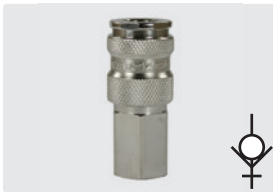
Coupling : F. Nickel-plated brass. With valve. Max. 35 bar / 100 °C
