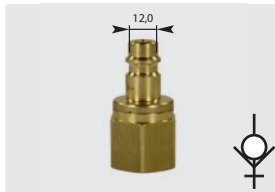
Plug : F. \varnothing 12 mm. Brass. With valve. Max. 35 bar / 100 °C
