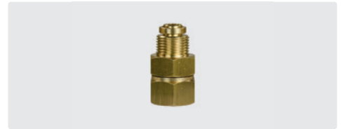
3/8" AG : 1/4" IG. Messing. Max. 220 bar / 90 °C
