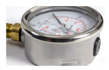
...that after the installation / assembly of pressure gauges filled with glycerine, a small opening must be pierced in the plug in the housing using a needle to ensure proper functioning? (Optionally, you can also use a paper clip or a pointed screwdriver to this end.)
