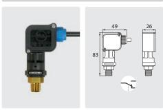
Contact 5 A - 250 V. Cable 950 mm. Thread 1/4" M. Max. 250 bar / 90 °C
