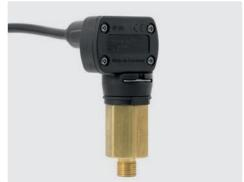
Contact 10.1 A - 250 VAC. Cable 950 mm. Max. 300 bar / 90 °C. IP65
