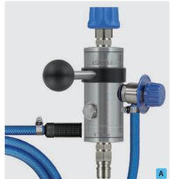
Coupling ST-45-250 nickel-plated brass: plug ST-45-250 stainless steel. Injector ST-167 with metering valve ST-161, suction hose 2,000 mm and suction filter ST-31. Max. 250 bar /  $100\,^{\circ}$ C
