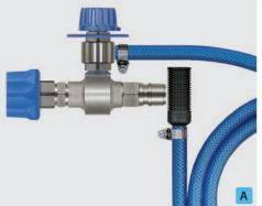
Coupling ST-45-250 nickel-plated brass: plug ST-45-250 stainless steel. Injector ST-160 with metering valve ST-161, suction hose 2,000 mm and suction filter ST-31. Max. 250 bar / 90  $^{\circ}$ C
