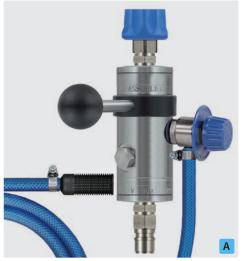
Coupling ST-45-250 nickel-plated brass: plug ST-45-250 stainless steel. Injector ST-167 with metering valve ST-161, suction hose 2,000 mm and suction filter ST-31. Max. 250 bar /  $100\,^{\circ}$ C
