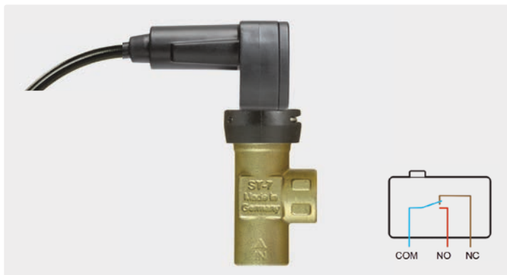
3/8" F. Protection class IP65. Cable 1,200 mm. 10 A. 250 V. Inrush current 20 A (NC) and 15 A (NO). Max. 350 bar / 45 l/min / 80 °C
