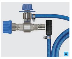
Coupling ST-45-250 nickel-plated brass: plug ST-45-250 stainless steel. Injector ST-160 with metering valve ST-161, suction hose 2,000 mm and suction filter ST-31. Max. 250 bar / 90  $^{\circ}$ C
