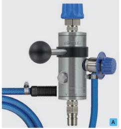
Coupling ST-45-250 stainless steel : plug ST-45-250 stainless steel. Injector ST-167 with metering valve ST-161, suction hose 2,000 mm and suction filter ST-31. Max. 250 bar /  $100\,^{\circ}$ C
