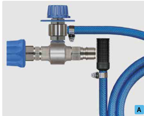
Coupling ST-45-250 stainless steel : plug ST-45-250 stainless steel. Injector ST-160 with metering valve ST-161, suction hose 2,000 mm and suction filter ST-31. Max. 250 bar / 90 °C
