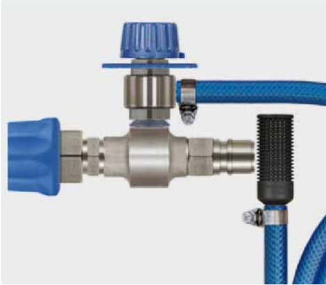
Coupling ST-45-250 stainless steel : plug ST-45-250 stainless steel. Injector with metering valve ST-161, suction hose 2000 mm and suction filter ST-31. Max. 250 bar / 90 °C
