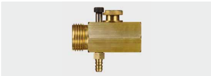
Injector with shiftable and disengageable chemical dosing. For suction of chemicals in the water inlet of the pump. Mixtures of chemicals/water can be applied by high pressure. Please use the backflow preventer (R+M Nr. 734 10). Hose tail 6 mm. Max. 10 bar / 90 °C
