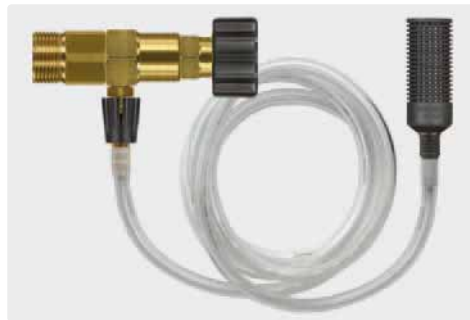
Injector with metering valve, suction hose 1000 mm and suction filter ST-31. Max. 220 bar / 90 °C
