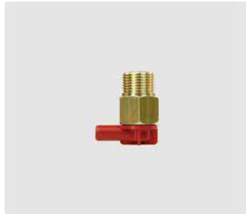
3/8" M : hose tail 6 mm. Valve with copper sonde. Working temperature 63 °C. Max. 10 bar
