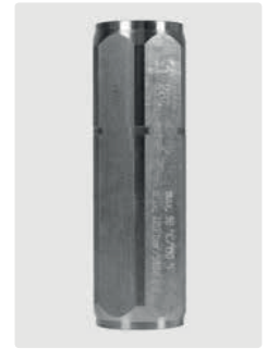
1/2" F. Stainless steel. [i] 90 mm. Opening pressure 0.05 - 0.1 bar. Max. 400 bar / 90 °C
