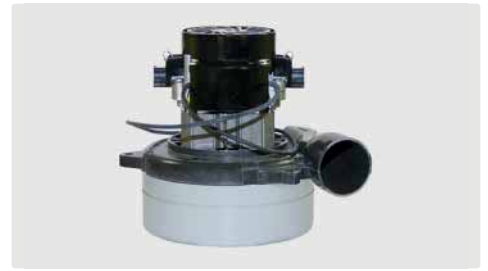
2 stage with waste air pipe. 24 V. Cable pre-installed
