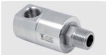
DGE 90°. Housing nickel-plated brass. Single ball bearing system. Rust-proof. Max. 275 bar
