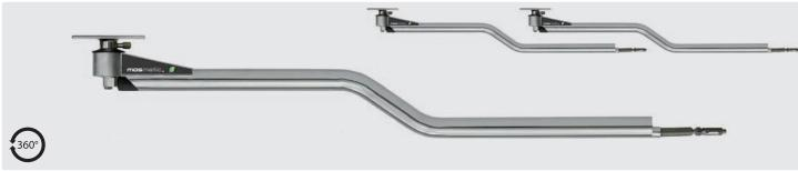
Stainless steel. Ready for installation with two integrated swivels. Especially designed for using two booms side by side. Insulated high pressure hose. Max. 275 bar / 90 °C.
