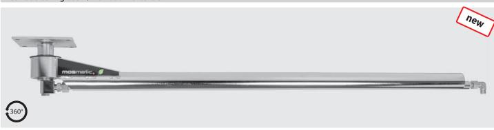
Stainless steel. This classic, straight ceiling boom is used in numerous industrial areas, such as truck washing, food, manufacturing or assembly. A real all-rounder that can be used in many ways. For the use of liquids, gases or air. 1/2" throughout. Max. 275 bar / 120 °C.
