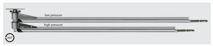
Stainless steel. Ready for installation with three integrated swivels, professional high pressure hose with spring and integrated hose bend restrictors. Axle 2-ball bearings and permanently lubricated. Especially developed for 2 different application mediums. Max. 275 bar / 90 °C.
