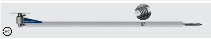
Stainless steel. Ready for installation with two integrated swivels and professional high pressure hose with spring and integrated hose bend restrictors. Axle 2-ball bearings and permanently lubricated. Max. 275 bar /  $90\,^{\circ}$ C.
