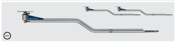
Stainless steel. Ready for installation with two integrated swivels and professional high pressure hose with spring and integrated hose bend restrictors. Axle 2-ball bearings and permanently lubricated. Especially designed for using two booms side by side.
