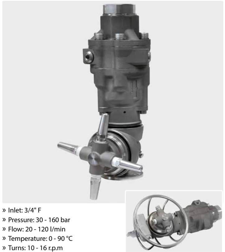
ST-82 h16/120 self rotating tank cleaner
