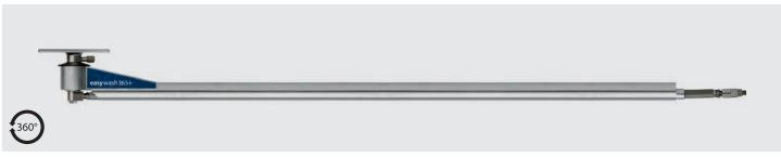
Stainless steel. Ready for installation with two integrated swivels and professional high pressure hose with spring and integrated hose bend restrictors. Axle 2-ball bearings and permanently lubricated. Max. 275 bar / 90  $^{\circ}$ C.
