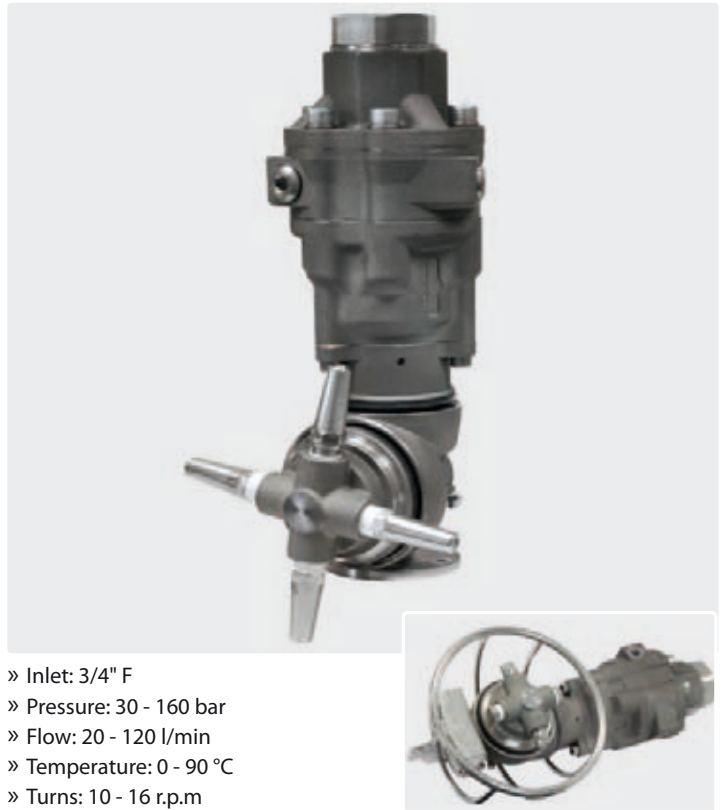
ST-82 h16/120 self rotating tank cleaner
