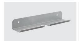
Stainless Steel. H x W x D 35 x 245 x 45 mm. Predrilled mounting holes at a distance of 190 mm
