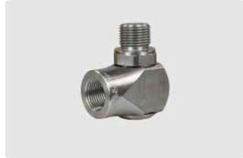
3/8" IG : 3/8" AG. DN 6. Max. 400 bar / 30 U/min / 90 °C
