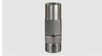
1/4" F : M22 M. Stainless steel. Swivel with radial friction bearing. Max. 350 bar / 90 °C
