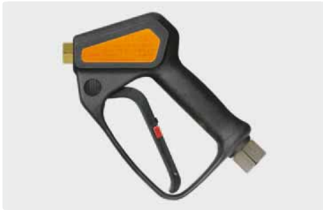
Professional gun. Max. 150 bar / 80 l/min / 150 °C
