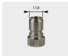
Plug : F. Stainless steel. Max. 250 bar / 150 °C
