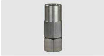
1/4" F : 3/8" F. Stainless steel. Swivel with radial friction bearing. Max. 350 bar / 90 °C
