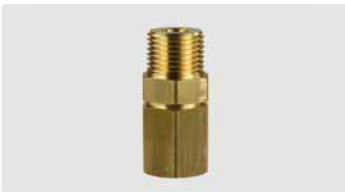
1/2" AG : 1/2" IG. Messing. Max. 250 bar / 90 °C
