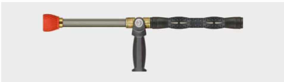
1/4" M. Longcast lance 500 mm with vented handle ST-9.1 260 mm, grip aside and nozzle protector made of plastic without nozzle. Max. 180 bar / 130 l/min
