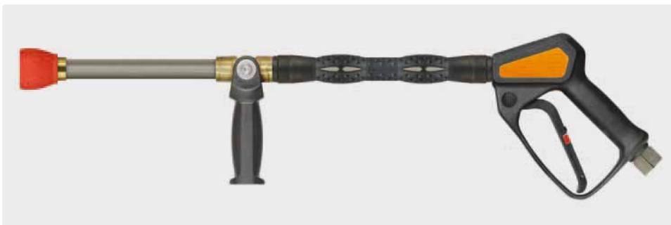
1/2" F. Longcast lance 500 mm with vented handle ST-9.1 260 mm, gun ST-2320, grip aside and nozzle protector made of plastic without nozzle. Max. 150 bar / 80 l/min
