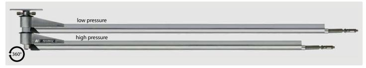
Stainless steel. Ready for installation with three integrated swivels, professional high pressure hose with spring and integrated hose bend restrictors. Axle 2-ball bearings and permanently lubricated. Especially developed for 2 different application mediums. Max. 275 bar / 90 °C.
