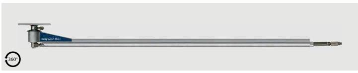
Stainless steel. Ready for installation with two integrated swivels and professional high pressure hose with spring and integrated hose bend restrictors. Axle 2-ball bearings and permanently lubricated. Max. 275 bar / 90 °C.
