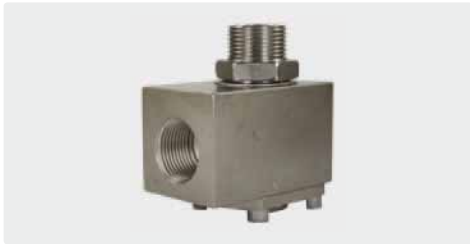
3/4" F : 3/4" M. Housing and axle stainless steel. DN 19. Max. 200 bar / 90 °C
