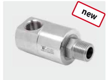
DGEI 90°. Housing stainless steel. Triple ball bearing system. Max. 350 bar
