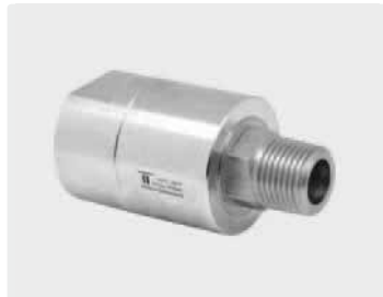
DGE. Housing nickel-plated brass. Single ball bearing system. Rust-proof. Max. 275 bar
