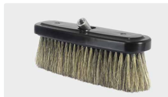
A= 260. B= 230 x 80 mm. Hog hair. With stainless steel frame. Max. 50 °C
