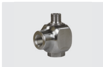
3/8" F : 3/8" M. DN 10. Max. 30 tr/min / 90 °C
