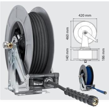
Hose reel: Base frame stainless steel V2A / AISI 304. Reel made out of especially impact-resistant ABS plastic with automatic spring-drive and traction release. Suttner swivel ST-322 made out of stainless steel. Max. 90 °C
