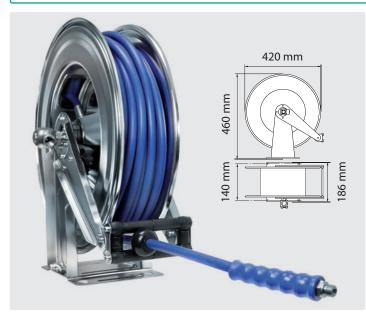
Hose reel: Stainless steel V2A / AISI 304. With automatic spring-drive and traction release. Suttner swivel ST-322 made out of stainless steel. Max. 90 °C
