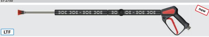
Professional ultra high pressure gun with patented LTF and lance with insulation ST-9, side handle and nozzle protector ST-10 without high pressure nozzle. Max. 500 bar / 30 l/min / 150 °C
