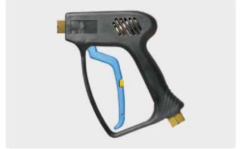
Professional gun. Weep version. Max. 275 bar / 45 l/min / 150 °C
