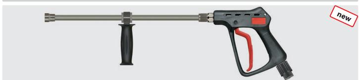
Professional ultra high pressure gun with lance 500 mm with grip and sleeve 1/4" F NPT stainless steel without high pressure nozzle. Max. 600 bar /  $150\,^{\circ}$ C
