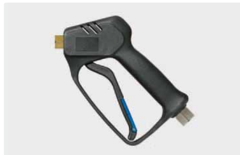
Professional gun. Weep version. Max. 210 bar / 25 l/min / 150 °C
