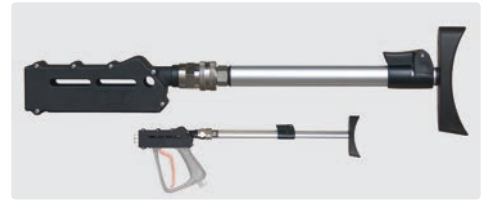
ST-3900 shoulder supports. New European Union guidelines imperatively prescribe the use of shoulder supports for cleaning applications exceeding an operating reaction force of 150 N. Variably adjustable ST-3900. Swiveling coupling. Suitable for guns ST-3600 / ST-3500.
