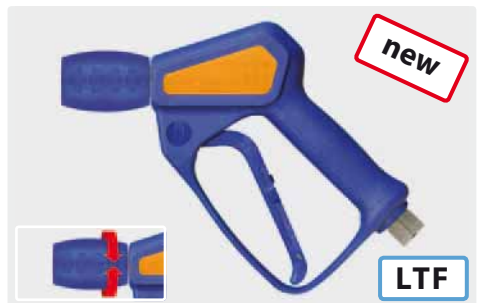
Professional gun with lance swivel ST-345. Freeze stop version. Max. 310 bar / 45 l/min / 150 °C
