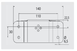
Stainless steel. Incl. fastening material for the injector.
