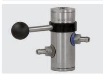
1/2" F: 1/2" F. Injector ST-168 with hose tail 9 mm and compressed air module (hose tail 9 mm). The chemical dosing is adjusted by 10 exchangeable nozzle inserts (0.5 - 2.0 mm). Max. 350 bar / 100 °C
