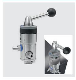
€ 3/8" F: € 1/2" F. Hose tail 9 mm. Injector ST-162 incl. 10 exchangeable nozzle inserts (0.5 - 2.0 mm) for regulation of chemical dosing. Improved foam characteristics due to symmetric air blow-in around the diffusor nozzle. Max. 350 bar / 100 °C
