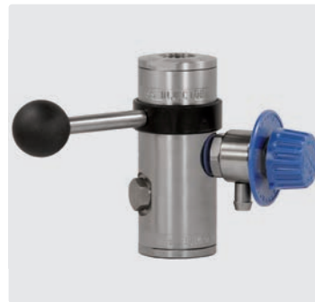
1/2" F : 1/2" F : hose tail 9 mm. Injector ST-167 with metering valve ST-161. Max. 350 bar / 100 °C
