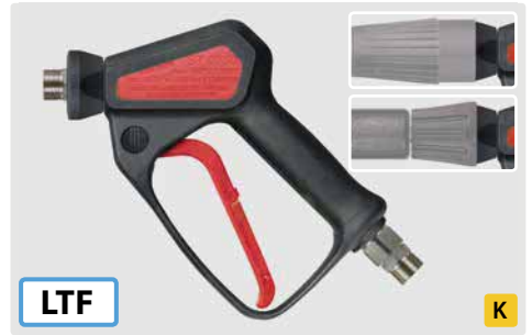
Professional ultra high pressure gun with patented LTF. Gun with insulated outlet suitable for lances with swivel screw coupling. Max. 500 bar / 30 l/min / 150 °C
